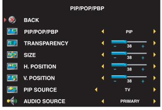
**NOTE:** You can use the PIP button or the POP/PBP button on the remote control to turn on and off PIP, POP, and PBP.
